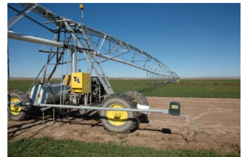
Low pressure linear sprinkler system
