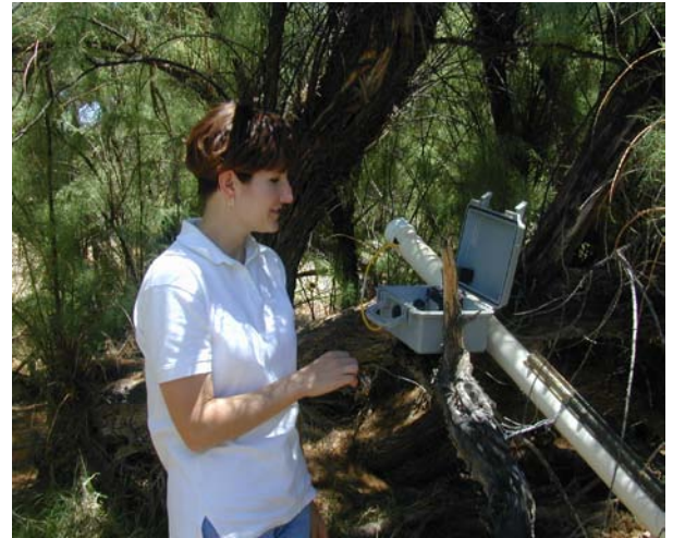
Alyson McDonald checking the water level logger on an untreated Salt Cedar stand
